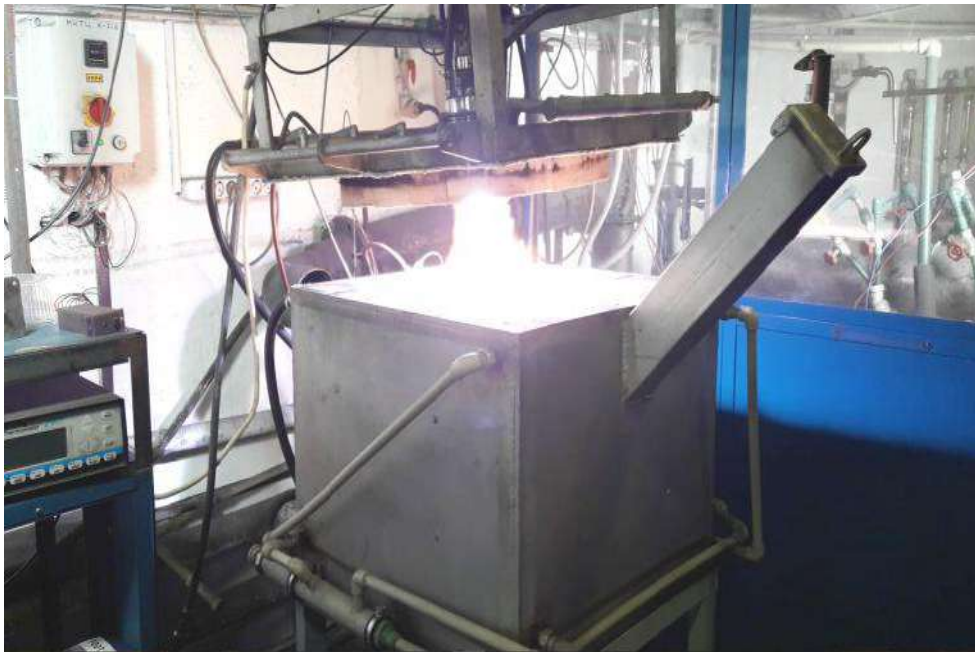
Figure 4 – Picture of the plasmatron in action with the reactor lid up
