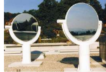
Figure7 Most heliostat are installed in rooftops, where there is plenty of space and sun exposure.
