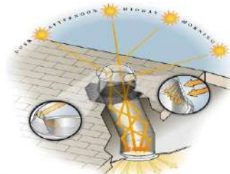
Figure2 The rooftop plastic dome collects the sunlight into the reflective tube to a ceiling-level diffuser.
